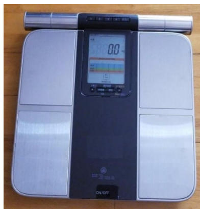
Fig. 4.10 Bioelectrical Impedance Analysis (BIA)
